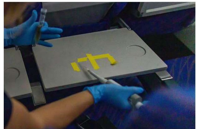
Virus is pipetted onto tray table for testing
