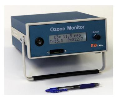
The 2B Technologies Model 202 Ozone Monitor™ is designed to enable accurate and precise measurements of ozone ranging from low ppb (precision of ~1.5 ppb) up to 250,000 ppb (250 ppm) based on the well-established technique of absorption of UV light at 254 nm. The Model 202 Ozone Monitor™ is lightweight (5.5 lb, 2.5 kg) and has a low power consumption (12V DC, 0.60 amp, ~7.2 watt) relative to conventional instruments and is therefore well suited for applications such as:
