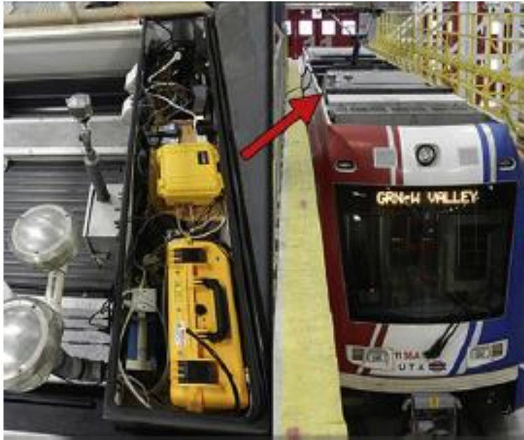
Air Pollution Instruments Installed on TRAX Cars
