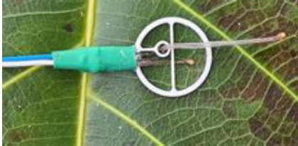
Leaf temperature sensor type LAT-B3, magnet-mounted on leaf surface.
