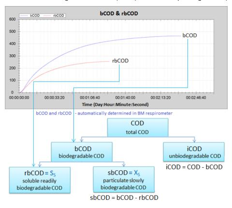
Many times the COD fractions can be determined by a single R test
