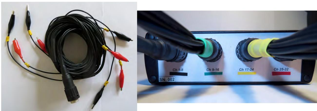
The package contains four electrode connection cables. Each of them includes 8 numbered crocodile clips with black and red colored endings. The main terminal should be connected to the back of the resistivity meter. Take care of connecting the right cable to the proper channels.
