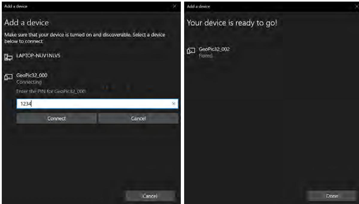
After pairing the resistivity meter, please check the COM ports at the “Device manager”.
