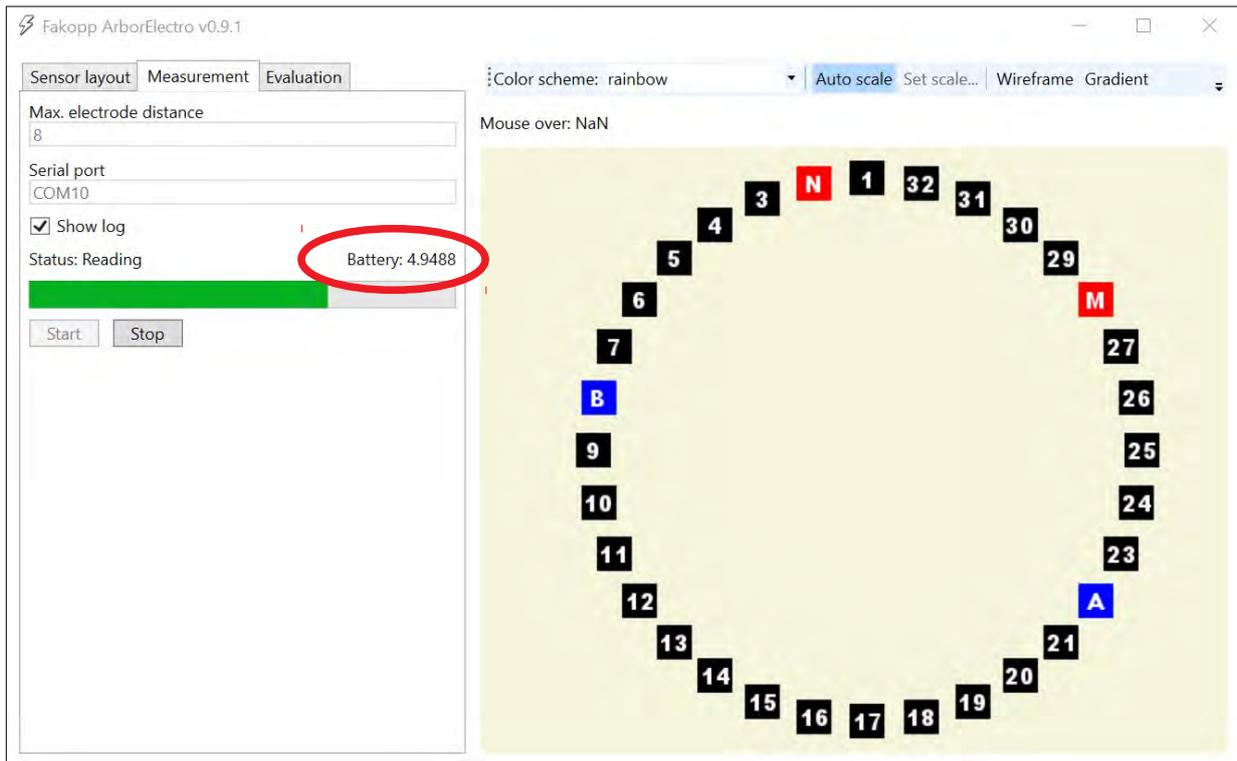
If the voltage output is under 4.94V it is recommended to charge the device. The current measurement can be finished and saved. But it is not recommended to start another one. The program sends you an error message in this case as well.
