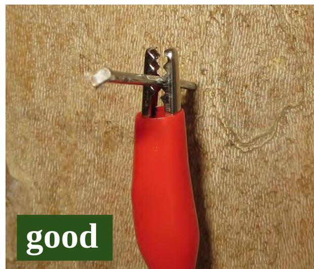
Be sure that the crocodile clips are on the needles, the needle is between the "teeth" and not under them.
