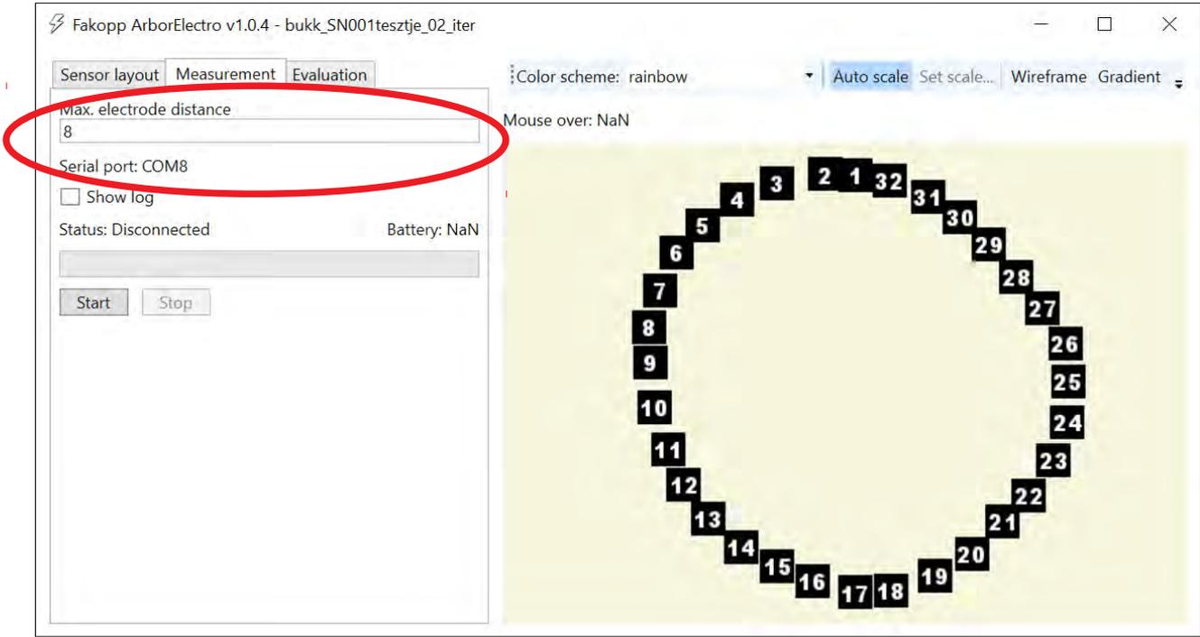
Max electrode distance is the biggest gap between two electrodes which has a role A, B, M or N. It is recommended to keep the maximal electrode distance offered by the program. Results can become unreliable if maximal electrode distance is too low (according to the number of used electrodes).
