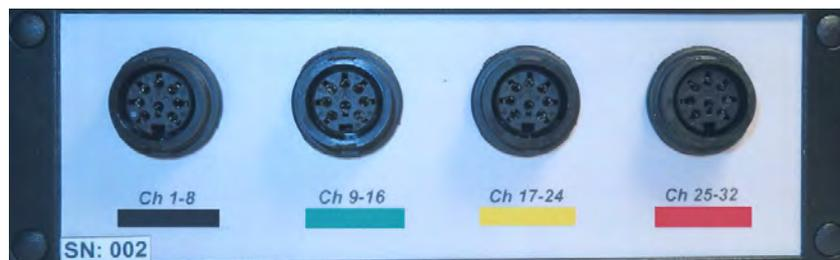
*The back of the GeoPic-32 Multielectrode Resistivity Meter
