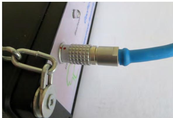
The cable connects the equipment to the computer. Use the blue end to connect it to the resistivity meter at the “USB” input. Look for the red dots for proper connection. The other end of the cable is a USB port, but it will be recognized as a serial port on the computer. (For more information about connection look for sub chapter First connection to computer.)
