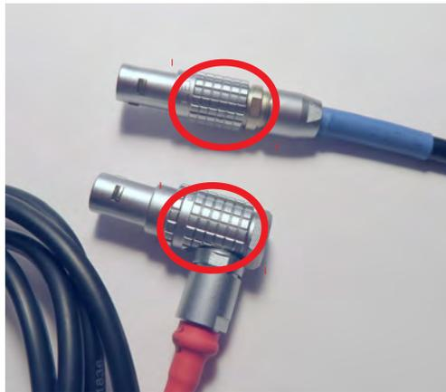
The LEMO ending has little “spikes” on it, please be careful when removing the cable from the device, please hold the vertical part.
