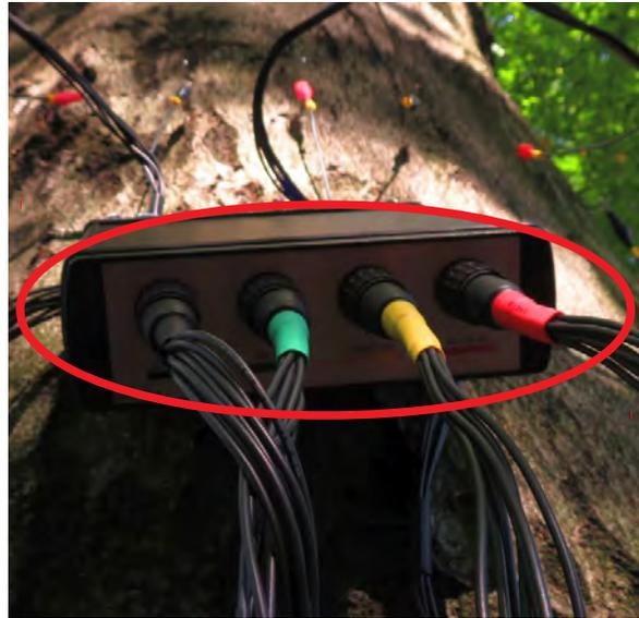
Connect the crocodile clips onto the electrodes. Start with the first electrode connection cable. Start with number 1 and go one by one till 8. The first clip is black. Please place it close to the resistivity meter. Use exactly one clip for one electrode. Do not skip an electrode or change the order.
