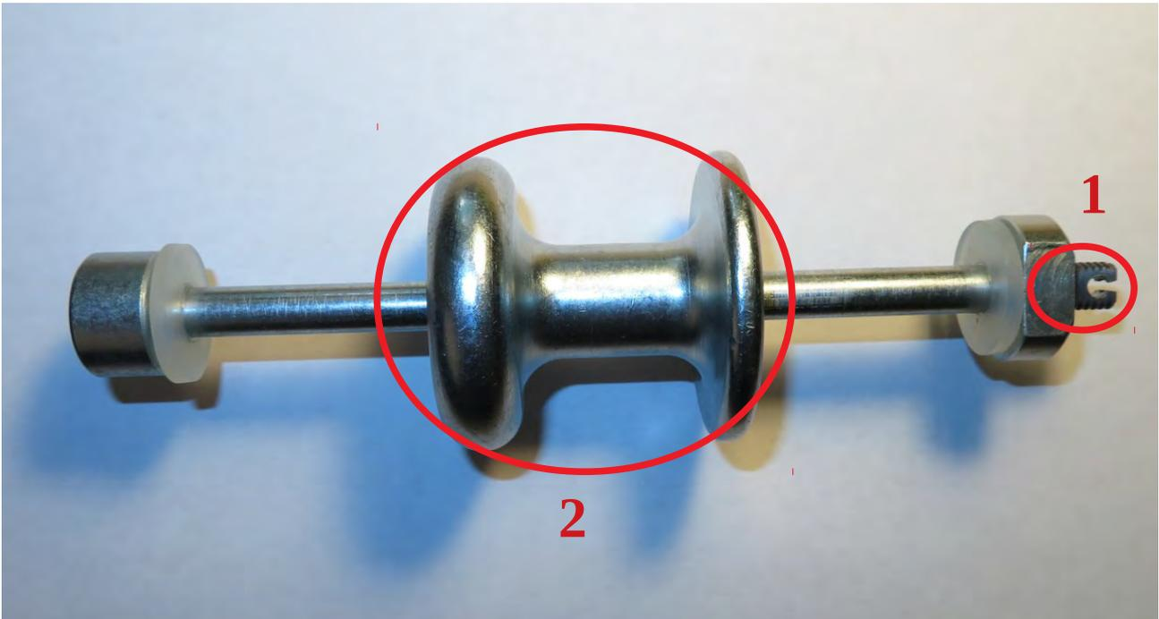
Electrodes can be easily removed by this electrode remover tool. Hold the tool as the end of the electrode is in the hole in one end (1). Then quickly push back the moving part (2) towards the other end of the tool. The push removes the needles serving as electrodes without bending them.
