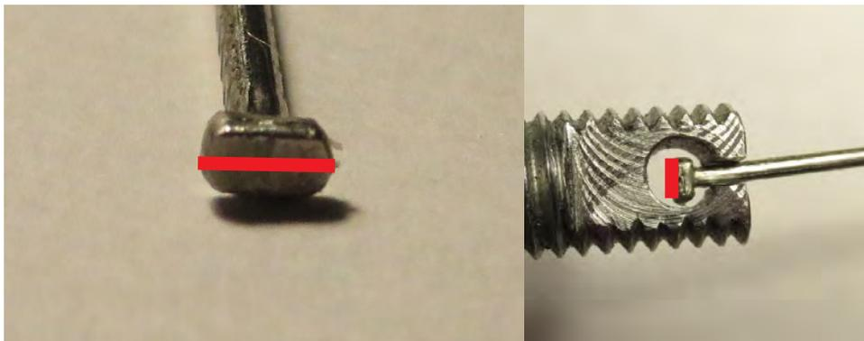
The head of the nails are rectangular. The electrode remover tool can be used only in the proper position.
