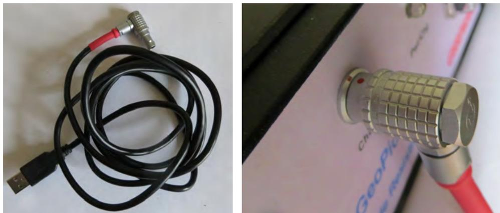
This cable connects the device to any USB ports or chargers for charging. The red end should be connected to the resistivity meter's "Charger" input. Look for the red dots to connect with the proper geometry.
