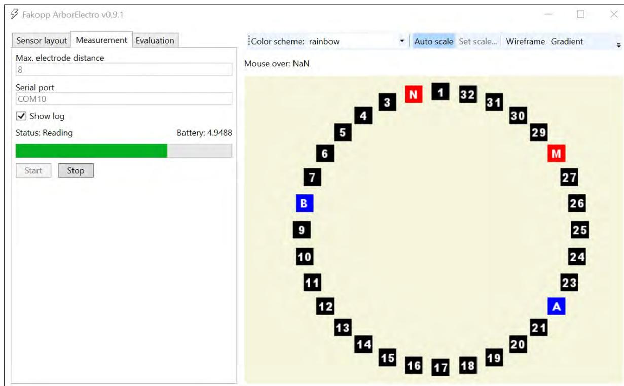
During the measurement you can follow how the roles of the electrodes are changing. A green status bar provides information about the progress of the measurement. It is possible to stop the measurement with pushing “Stop” button but in this case the previously measured data will be lost.
