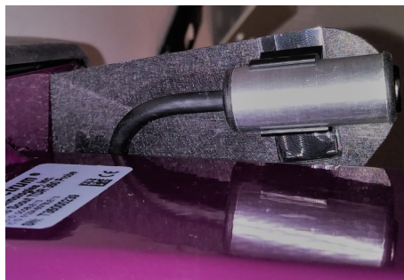
Fig. 5: IRT sensor attached to bracket
