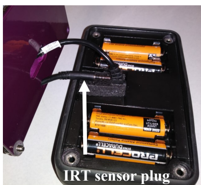
Fig. 2: IRT sensor inserted through flange
